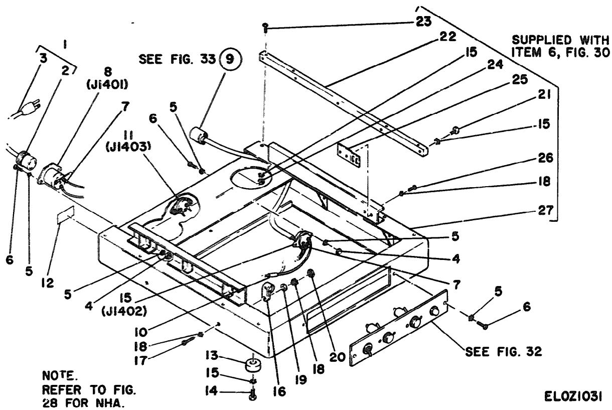
Figure 31 Cabinet assembly, lower
