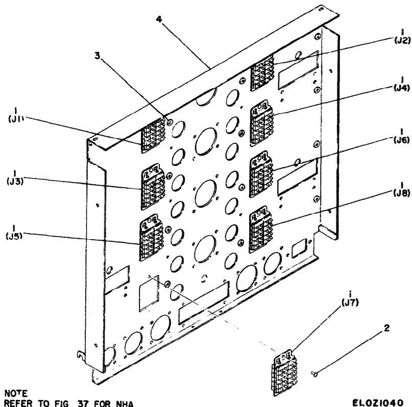
Figure 40 Chassis assembly 00356-63070
