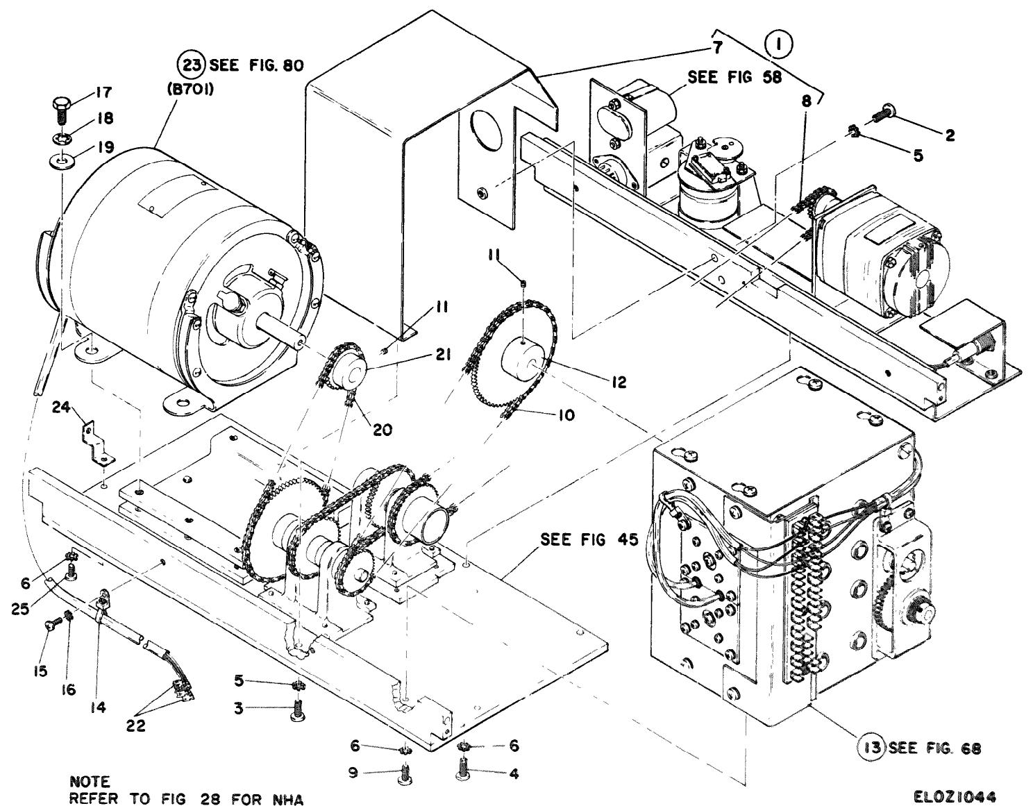
Figure 44 Motor gearbox
