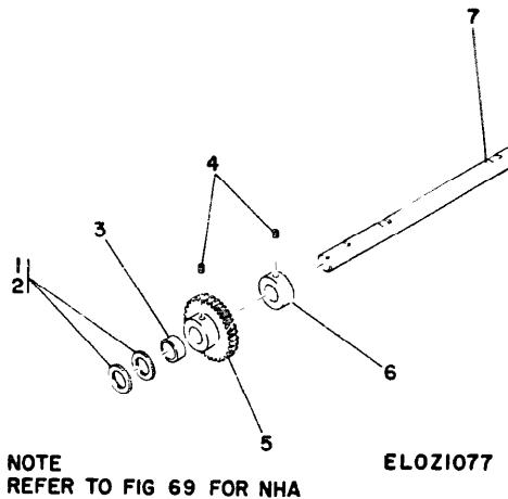
*Figure 77 Gear assembly (H)*
