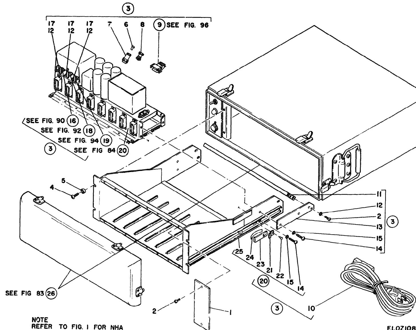
Figure 82 Subassembly for Power Supply AN/USM-365
