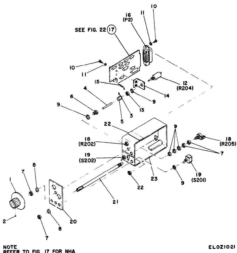
Figure 21 Plug-m unit for PL-1307/U
