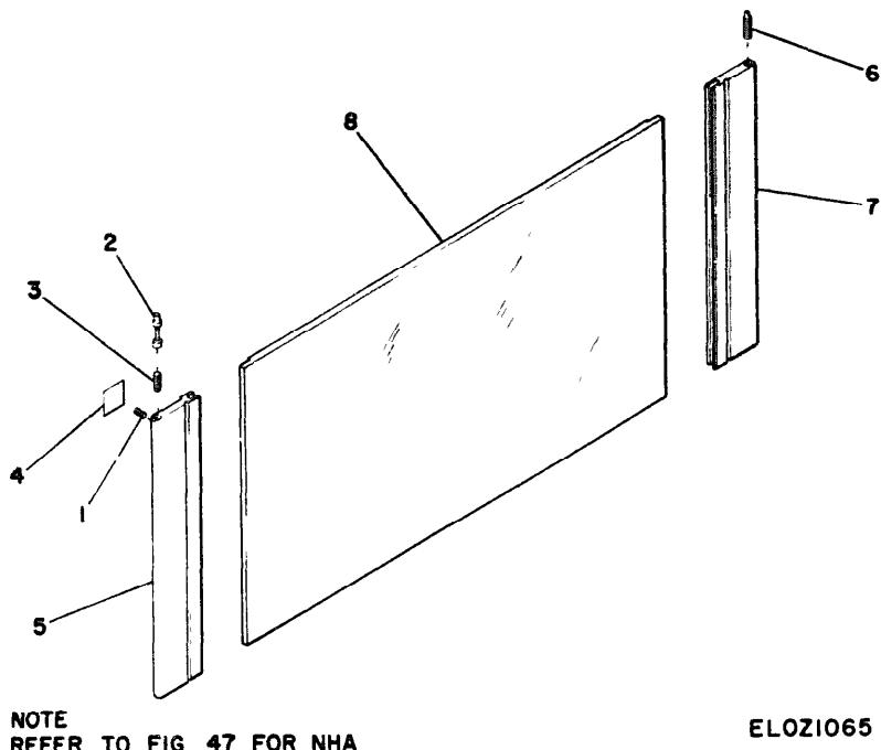
Figure 65 Door assembly access
