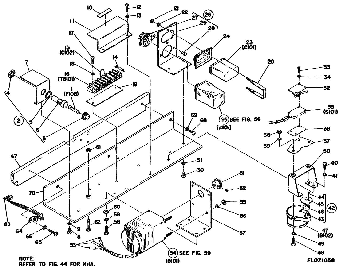
Figure 58 Motor drive kit.
