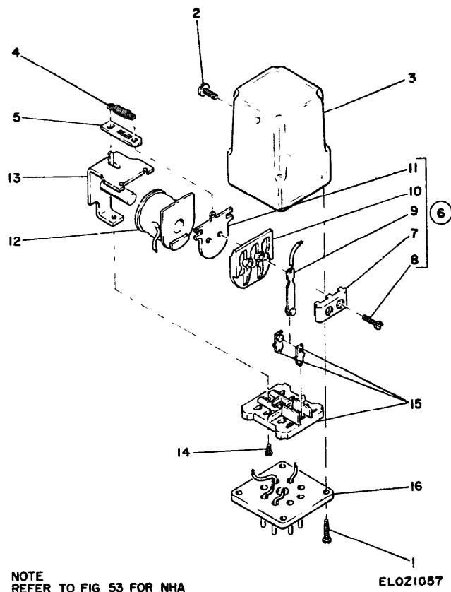
Figure 57 Relay armature 0490-0416
