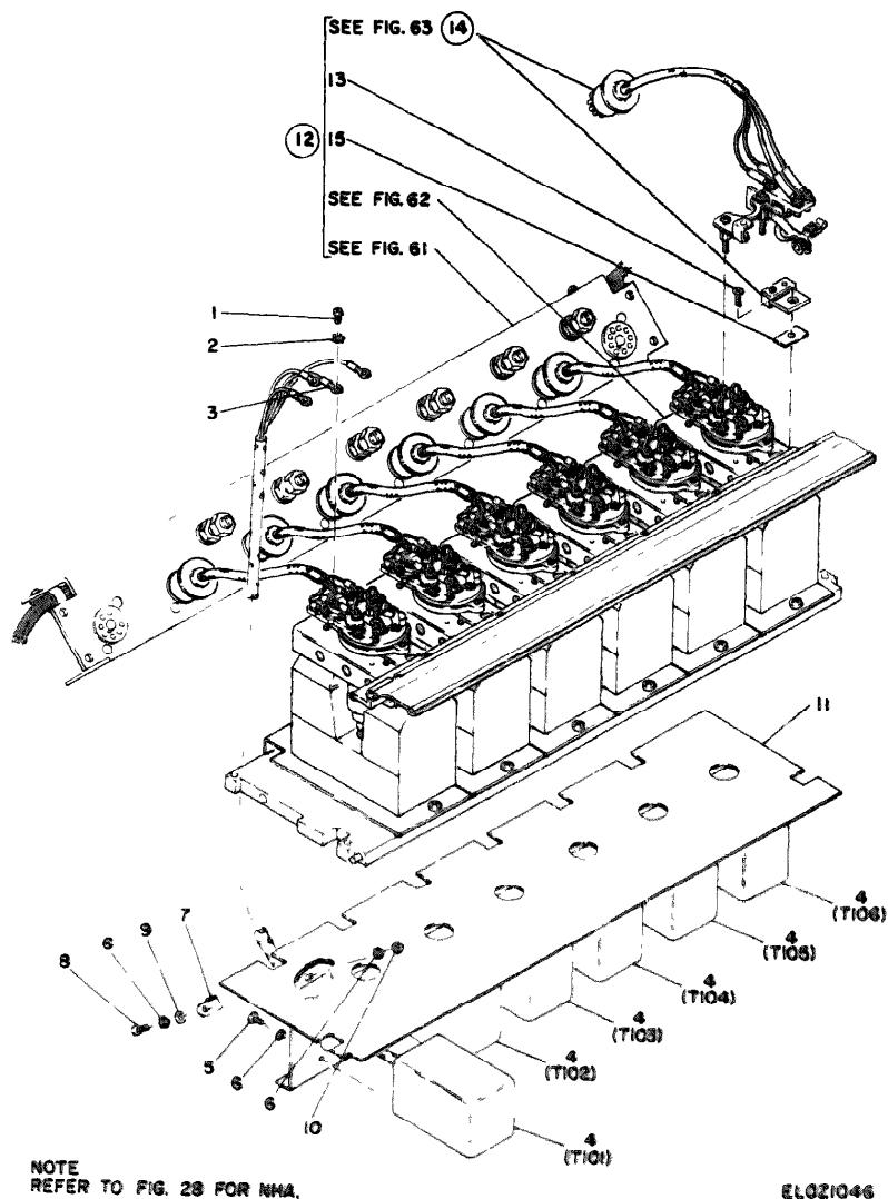
Figure 46 6-channel galanometer assembly
