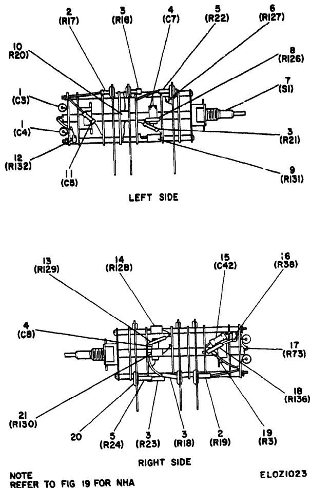
Figure 23 Switch assembly for PL-1307/U
