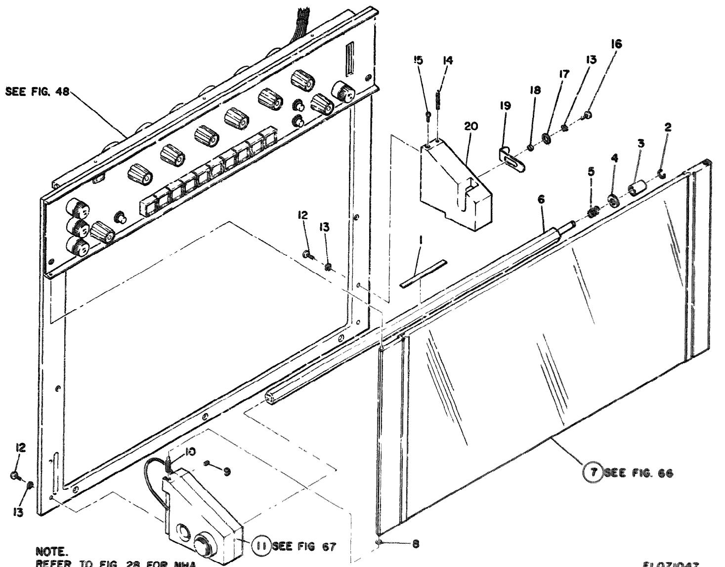
Figure 47 Front panel assembly (A)
