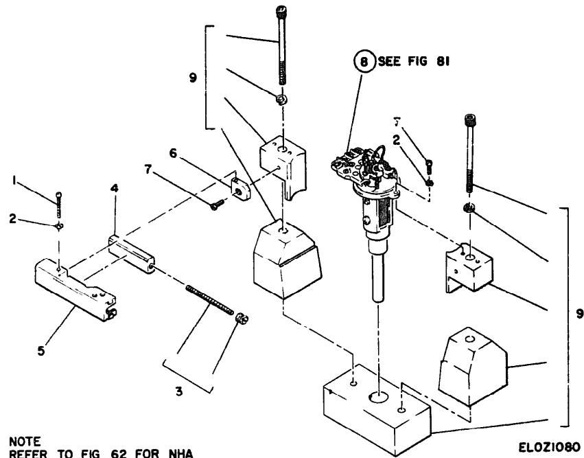
Figure 80 Galvanometer HP607A
