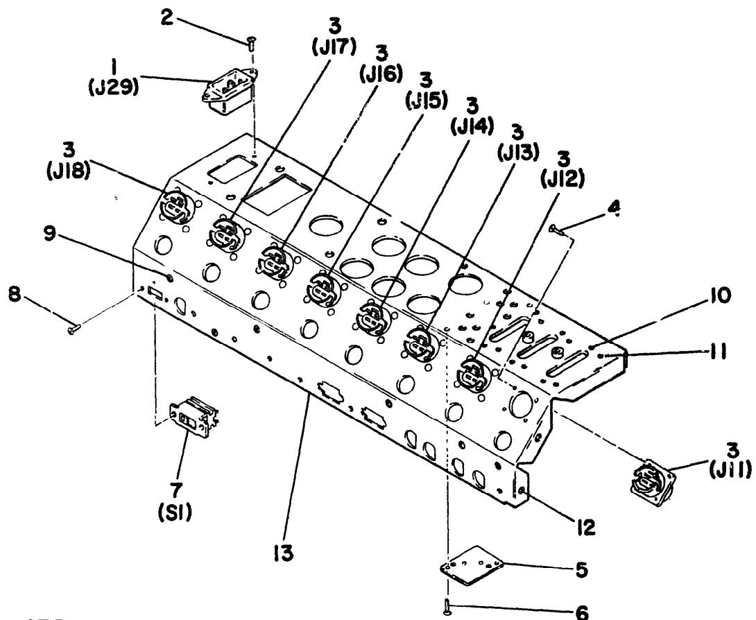
Figure 89 Power *supply frame*
