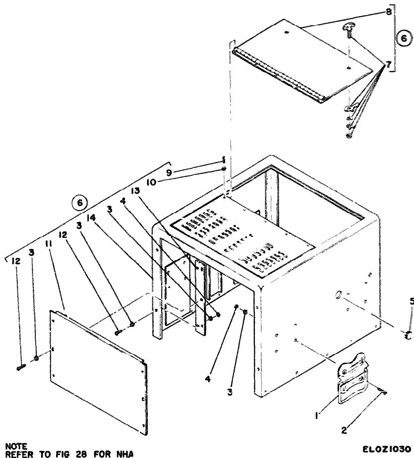
Figure 30 Cabinet assembly, electrical equipment
