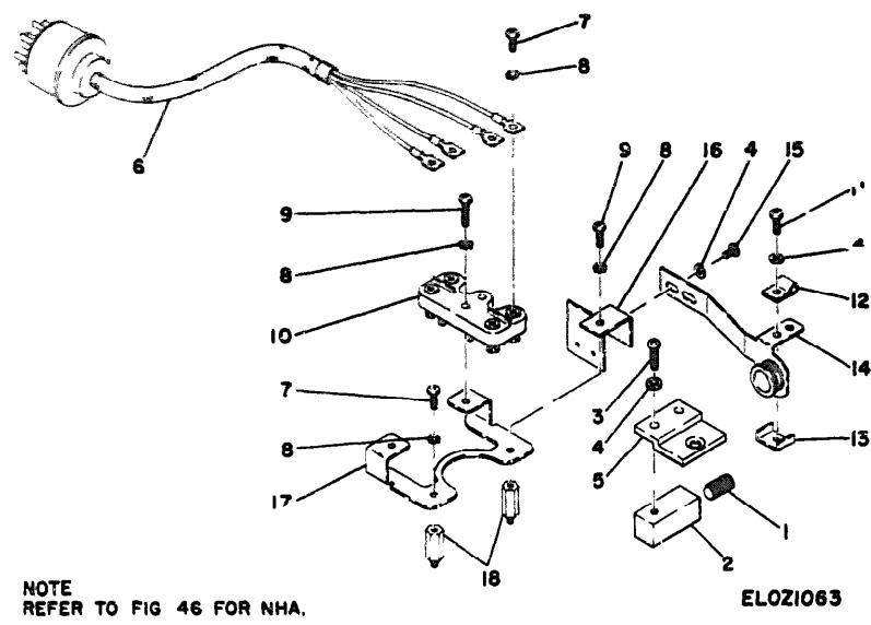
Figure 63 Galvanometer mounting
