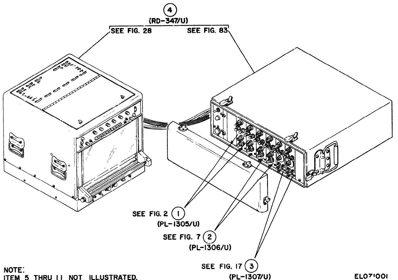
Figure 1 Recorder. Thermal Oscillograph AN/USM-365 (V)1
