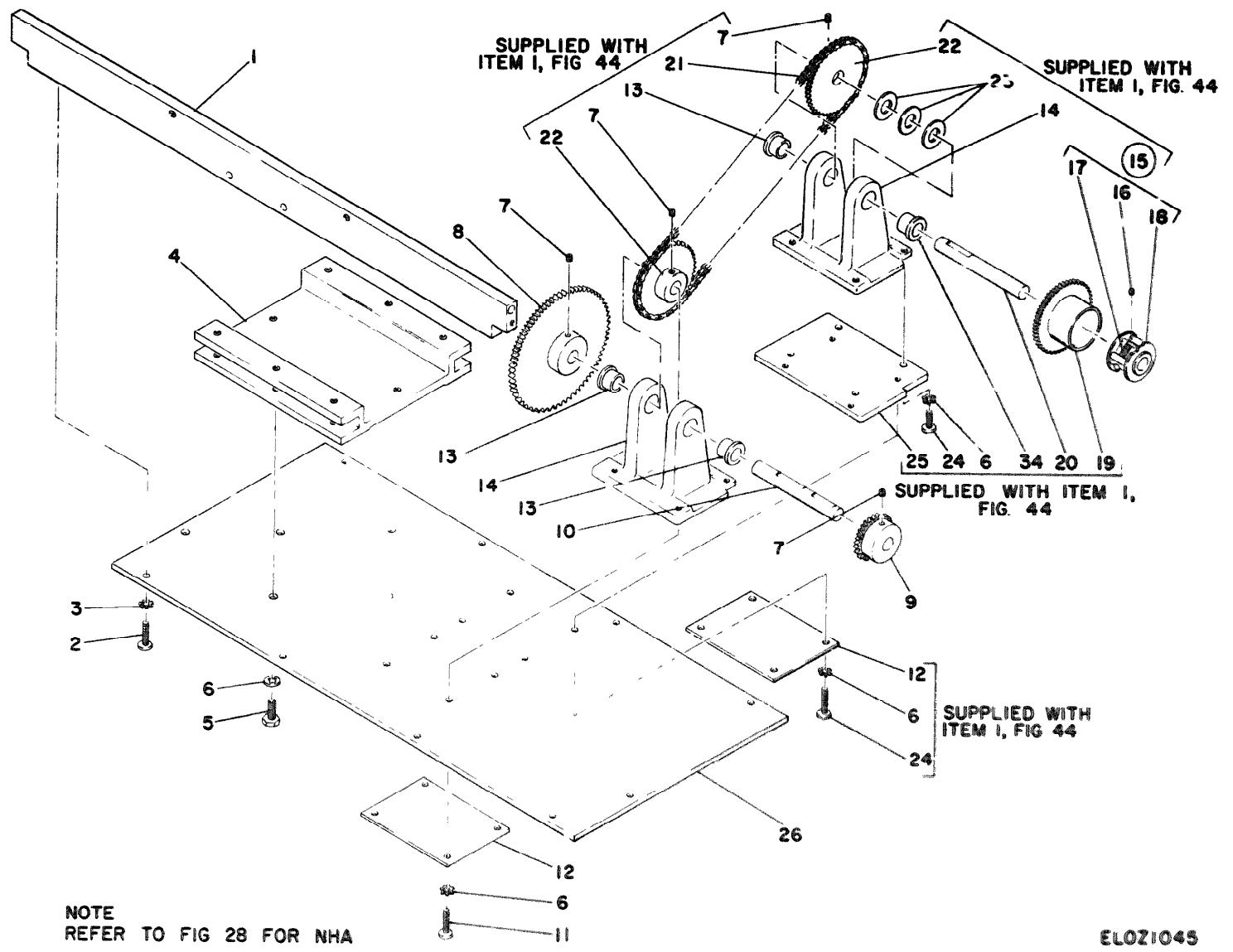
Figure 45 Motor gearbox bottom
