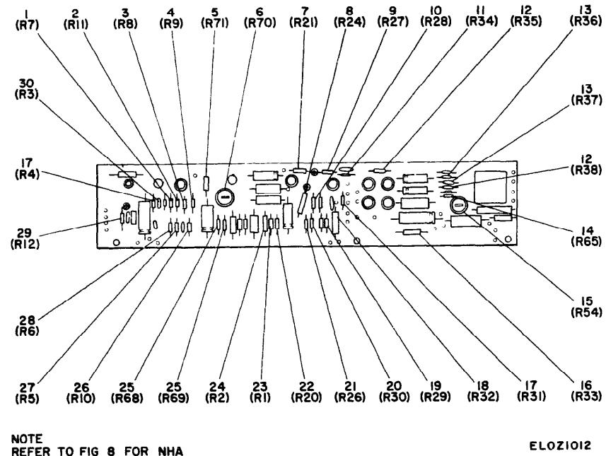
Figure 12 Circuit card assembly (B) for PL-1306/U
