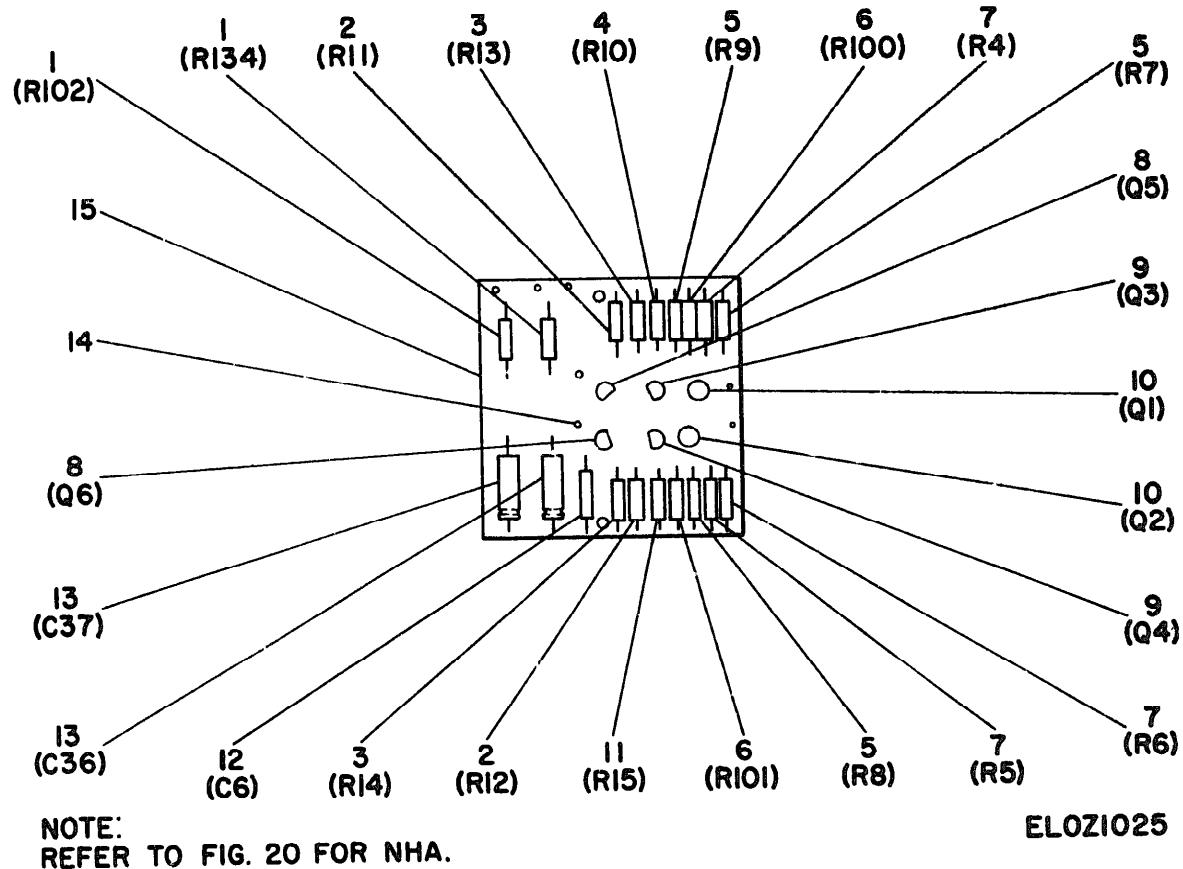
Figure 25 Circuit card assembly (B) for PL-1307/U
