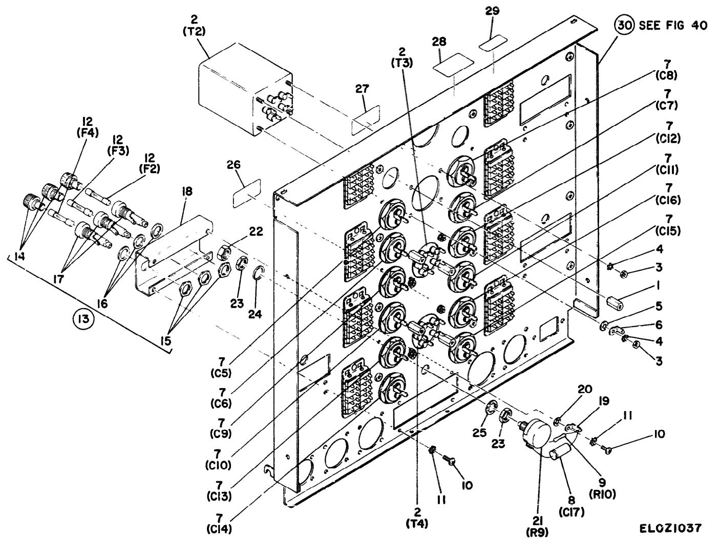
Figure 37 Power supply assembly (B).
