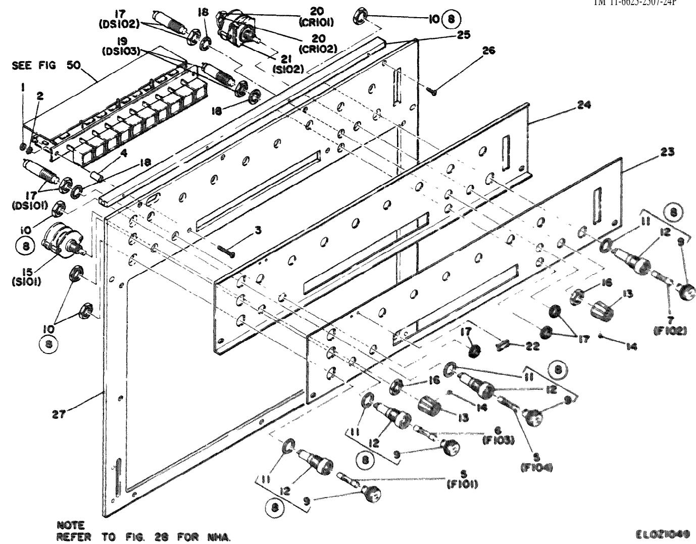
Figure 49. Front Panel, assembly (C)
