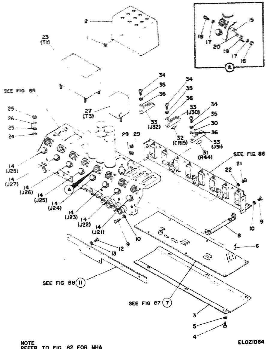
Figure 84 Power supply HP848A
