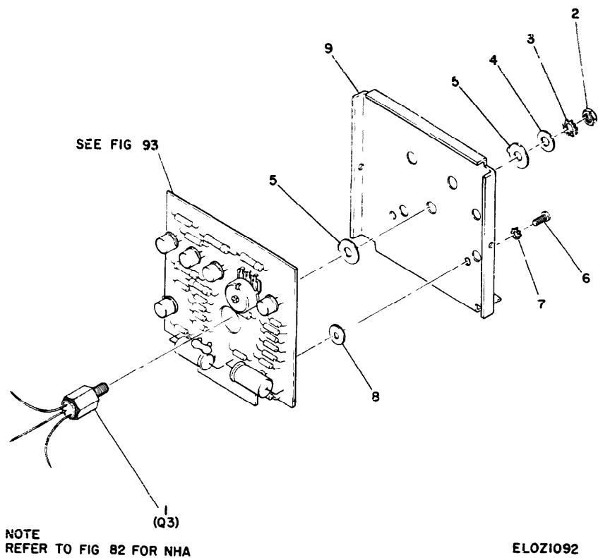
Figure 92 Circuit card assembly 868-500AC6
