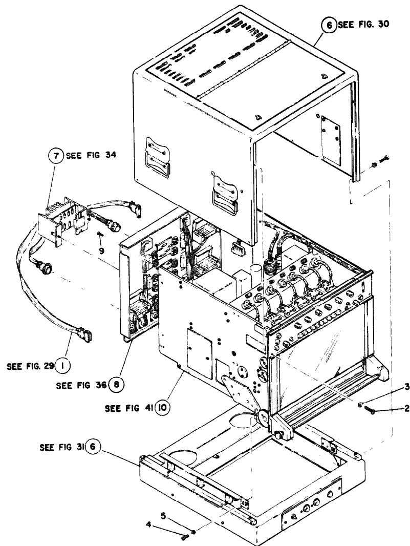
Figure 28 Oscilloscope Subassembly RD-247/U
