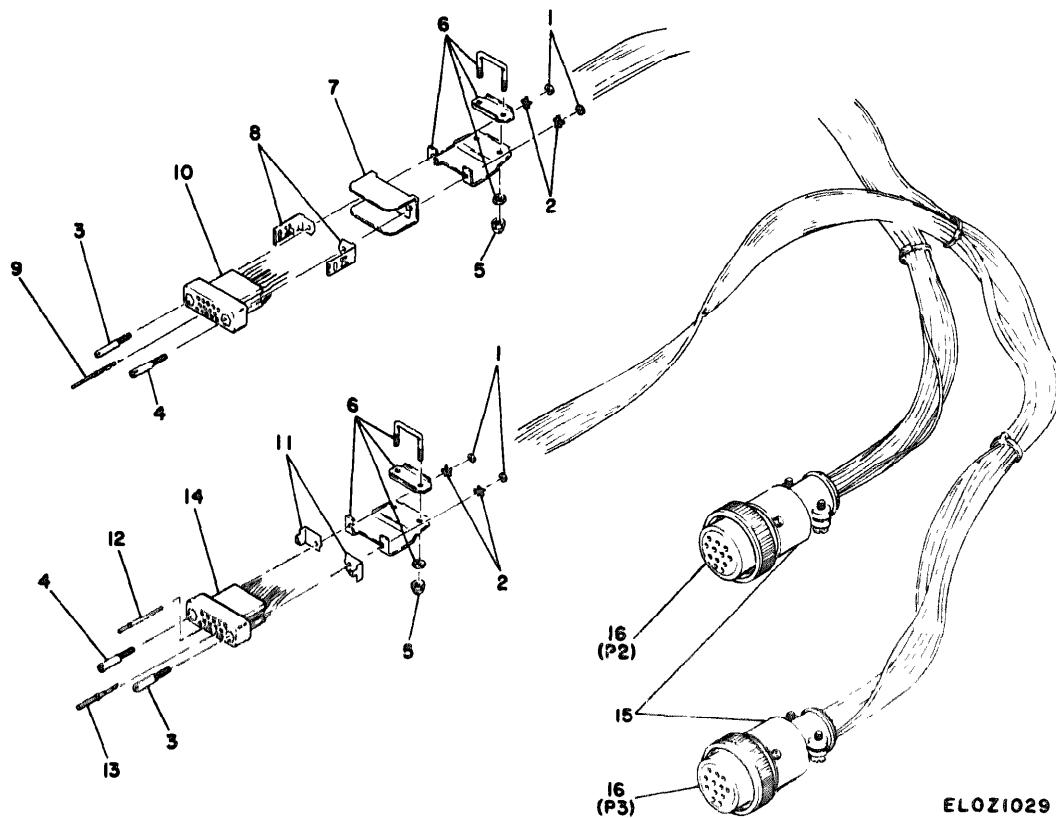
Figure 29 Cable assembly, special electrical
