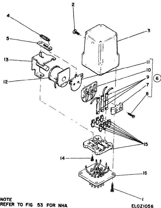
Figure 56 Relay armature 323D10-5
